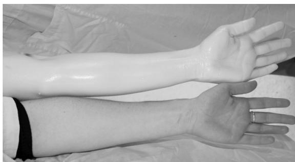
*Fig. 1: A three-dimensional, life-like bite target cast as a silicone replica from the impression (top) of an actual arm (bottom), fitted with a rigid bony interior.*
