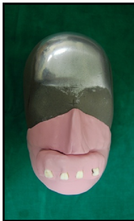
Fig. 1: Tooth mounting on crash test dummy head
